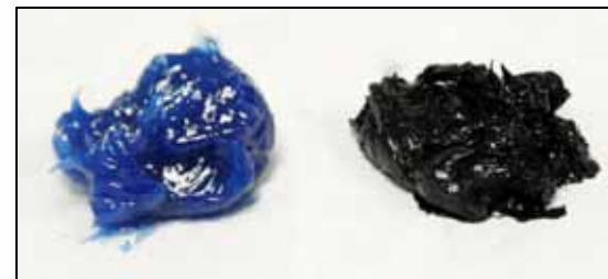
new grease vs burnt grease
