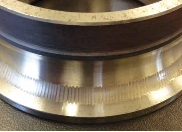
Fluting damage on bearings caused by induced currents passing through the bearings
