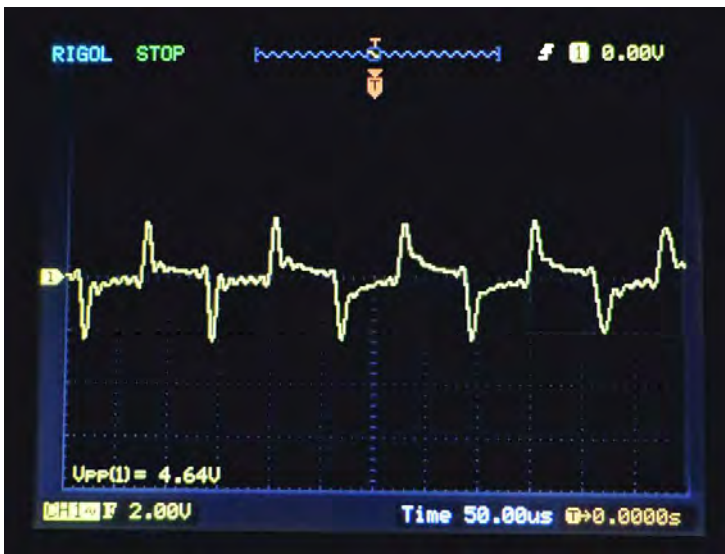
Shaft Voltage with Fiber Ring
